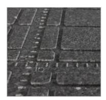
imprinted scale to facilitate the cutting of boards
